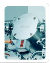
The positive displacement diaphragm pump provides pressure independent flow, ensuring critical parameters do not vary during concentration.
