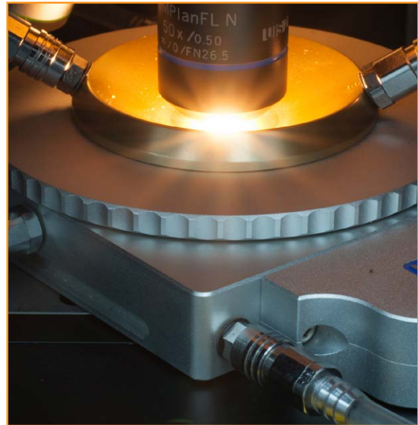
Using LiveTrack to maintain focus on the surface of a sample in a high temperature cell.
