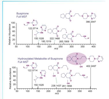
Full MS/MS spectra of busiperone, an anxiolytic drug, and a hydroxylated metabolite of busiperone. Assigned masses of identified fragments were all within 1 ppm of their theoretical values. High resolution, accurate mass, and outstanding spectral quality add Q Exactive confidence to metabolite studies and structural ID.
