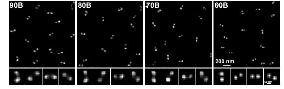
GATTA-STED Nanoruler 90B, 80B, 70B and 60B (GATTAquant, Germany) were imaged and processed with Elyra 7 Lattice SIM<sup>2</sup> mode with a 63×/1.4 oil objective. Distances of 90 nm, 80 nm, 70 nm and 60 nm are resolved.
